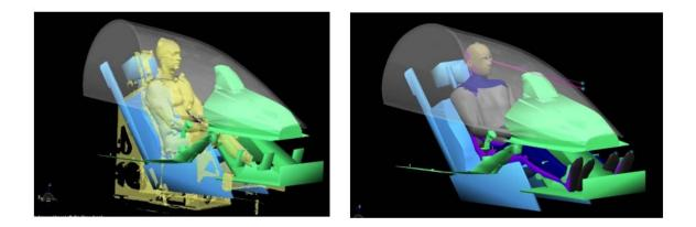
Sensors ensure a proper posture of the trainee at the ejection seat: head, shoulder left/right, elbow left/right and legs. Trigger button of firing is included in the safety chain. Pressure sensors, mechanical interlock of ejection cylinder for unintended firing. Emergency stop system, sledge/seat hold and descent device with safety damping cylinder.
