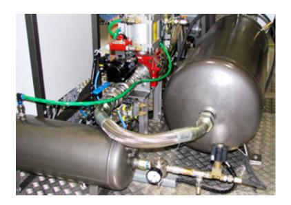
The pneumatic ejection system consists of a compressed air cylinder, an air charging system, a pressure regulator and pneumatic valves. Controlled by a PLC according to the required G-load and trainee's weight. Furthermore, the system is integrated in the safety system to prevent the occurrence of training emergencies.
