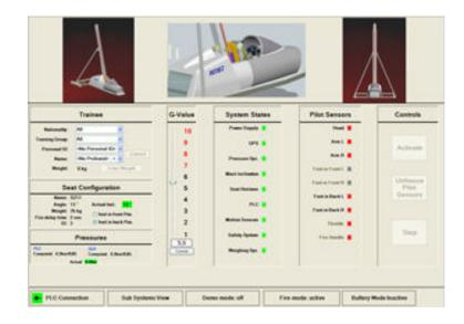
The **G-SENSOR MATRIX 1** control and monitoring system is the kernel software to guarantee safe and reliable system operation. The control computer implements all algorithms, which calculate the force profile (compressed air pressure) required for the required G-load and loading weight. The pneumatic system is fully automatically controlled and monitored.
