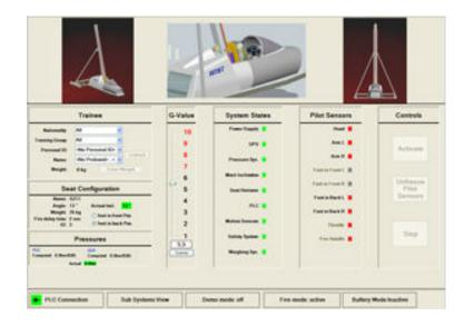
The **G-SENSOR MATRIX 2** control and monitoring system is the kernel software to guarantee safe and reliable system operation. The control computer implements all algorithms, which calculate the force profile (compressed air pressure) required for the required G-load and loading weight. The pneumatic system is fully automatically controlled and monitored.
